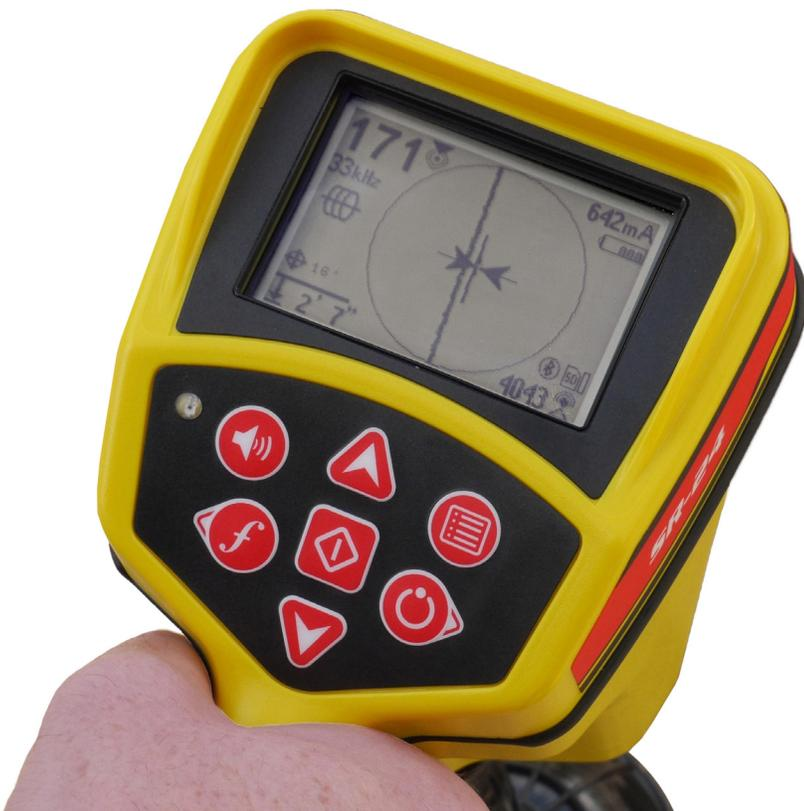
If you locate utilities with a more contemporary receiver, such as the RIDIGD® SeekTech® SR-24 receiver, you might be familiar with some version of the left-right arrows that show you the signal's position relative to the locator's. This boasts better accuracy than looking at signal strength alone. The more pieces of useful information you have about a signal, the better.
