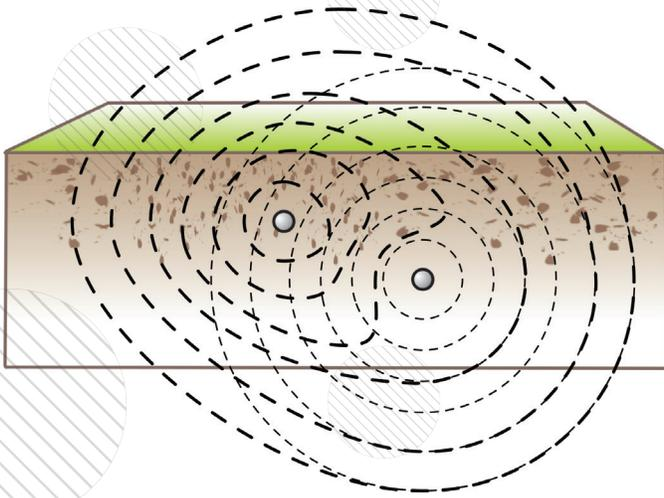
Interference from a nearby energized utility warps the signal shape and makes peak and null readings less reliable.
