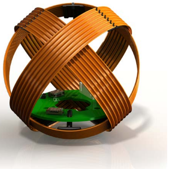
A cut-away of an omnidirectional antenna array showing the coil arrangement.
