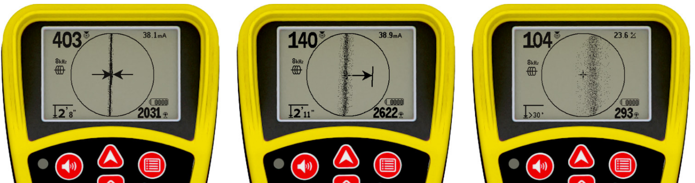
Omnidirectional receivers can indicate degrees of signal distortion. The fuzzier the tracing line is on the display, the more distorted the signal.
