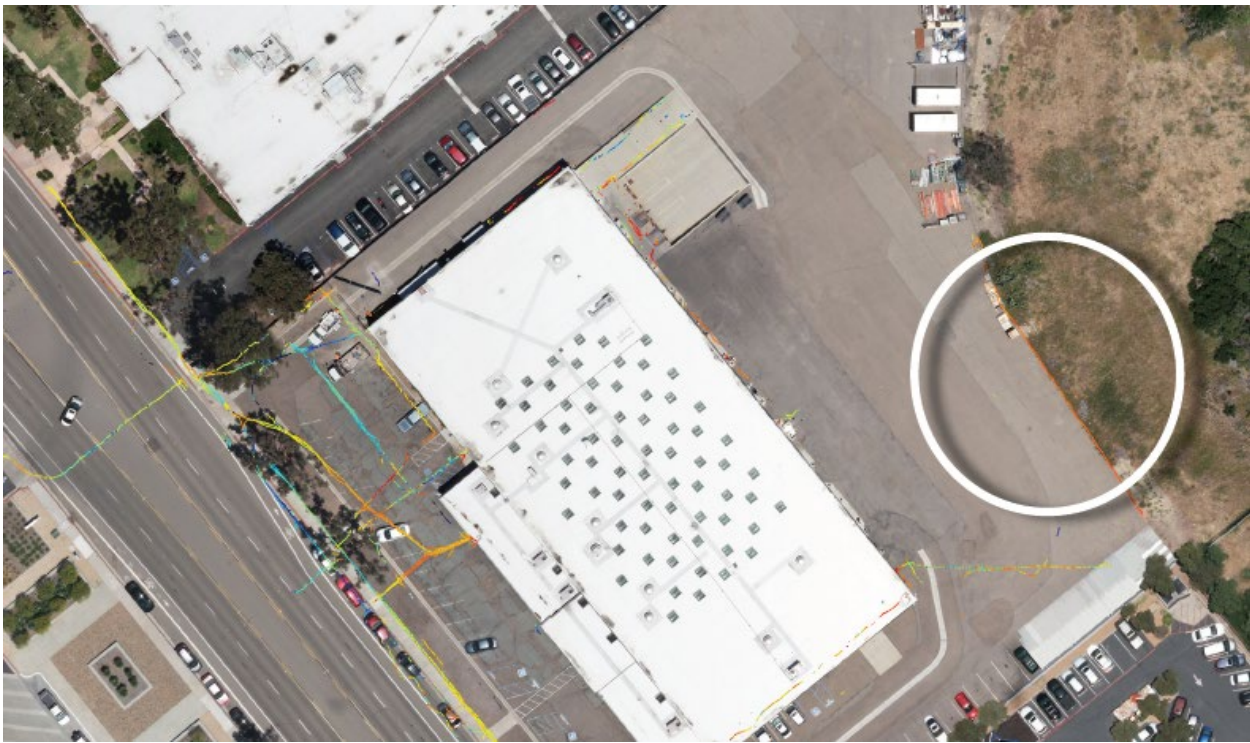
Figure 3 - The map data in SubView shows multiple distinct utilities throughout the front and back parking lots. A line running along the canyon edge reveals a separate utility energized via signal bleed.
